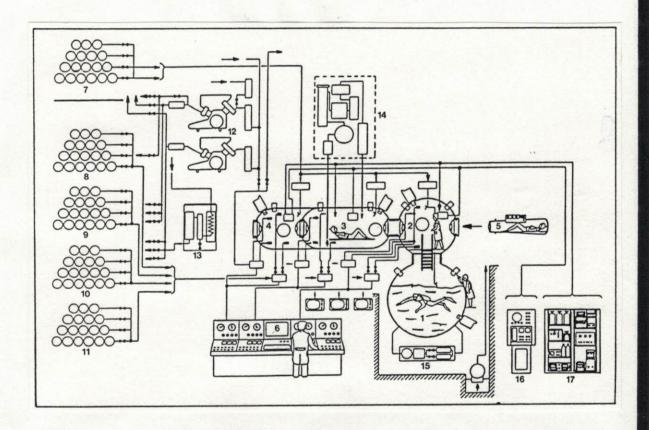
Fig. 2.15: schematic diagram of monitory-, supply-, and life-supporting systems and peripherals
