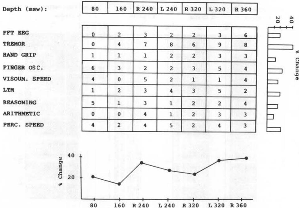
Fig. 5. Condensed data presentation of all tests indicating number of divers with an impairment of 2 SD or more. Lower curve indicates the general level of test impairment at the different depths. Curve at right indicates the relative impairment on the different tests during the compression. R = reach, L = leave.
