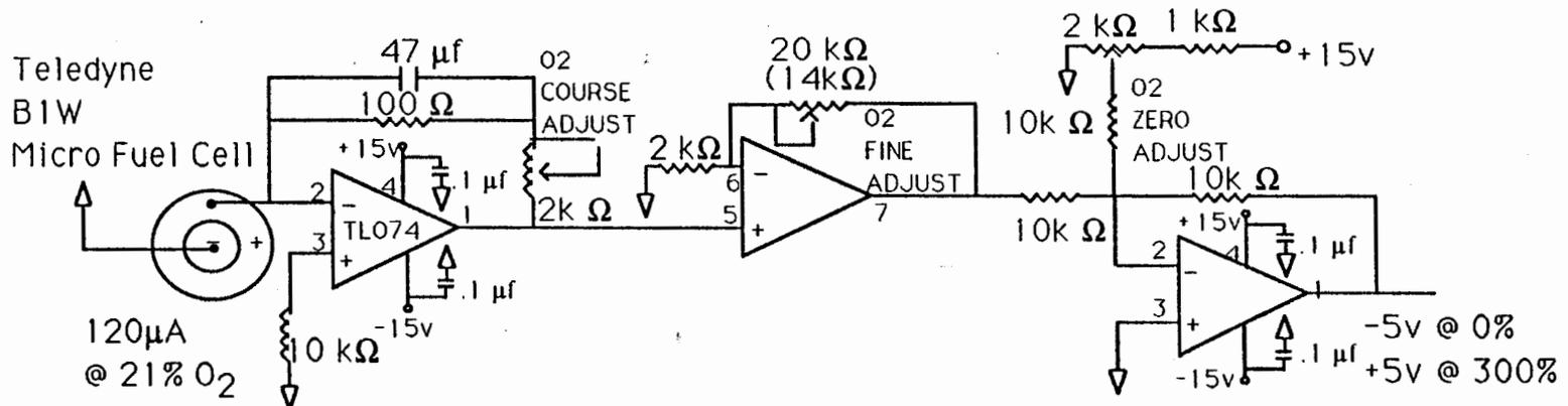
Figure 4: Amplifier circuit for Teledyne model B7W micro fuel cells used to determine oxygen partial pressures within the closed-circuit breathing apparatus.
