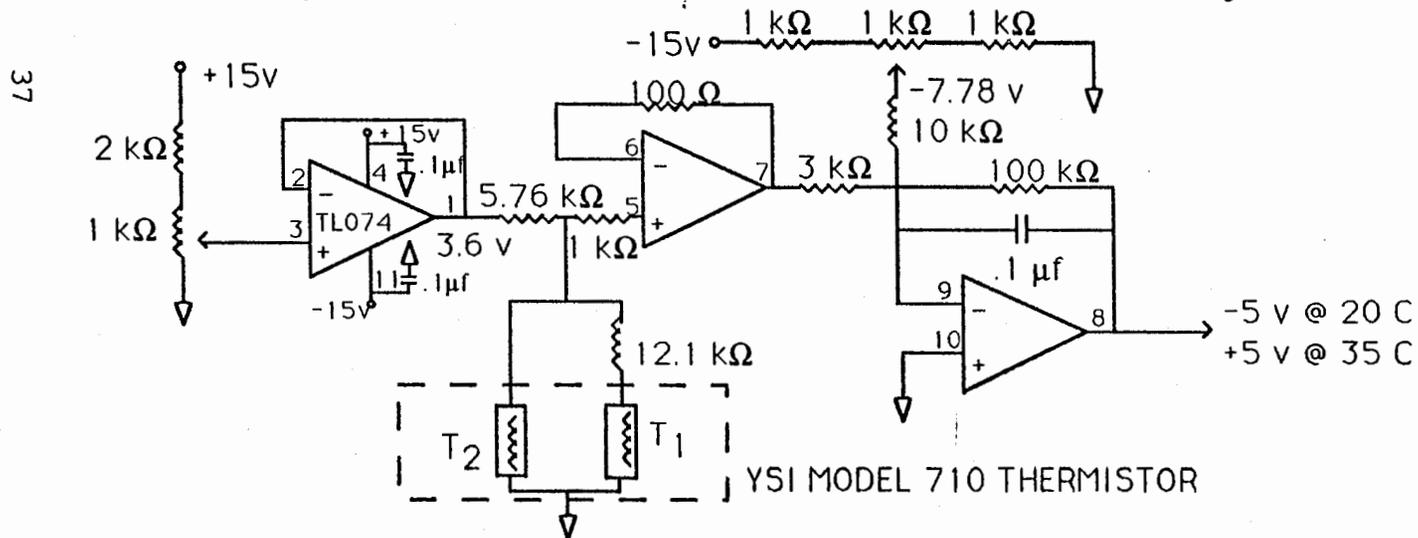
Figure 5: Amplifier circuit for YSI model 710 thermistor used to provide temperature compensation for volume and oxygen partial pressure determinations.
